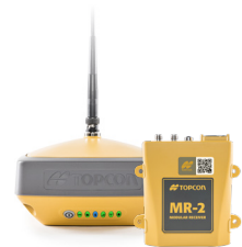
Correction Services Full range through base stations (HiPer VR and MR-2) and reference station networks (TopNET)
