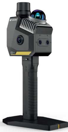
The Topcon CR-S2 combines MLF-SLAM (multiple localization fusion-SLAM), VSLAM (visual SLAM), and RTK-SLAM technologies. This integrated approach delivers stable, centimeter-level accuracy - even in areas where GNSS signals are weak or unavailable - by leveraging LiDAR, visual, IMU, and RTK data. High-fidelity point clouds and real-time colorized imaging ensure actionable results in a single workflow, minimizing return visits and rework.
