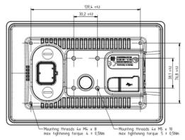
Note: dimensions are in millimeters (mm)
