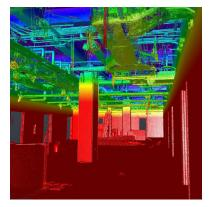
For renovations or improvement fit-outs, Young said they first scan all the existing conditions, then incorporate that scan data into the design models or provide it back to the design team to confirm that steel or existing systems are where they should be.
